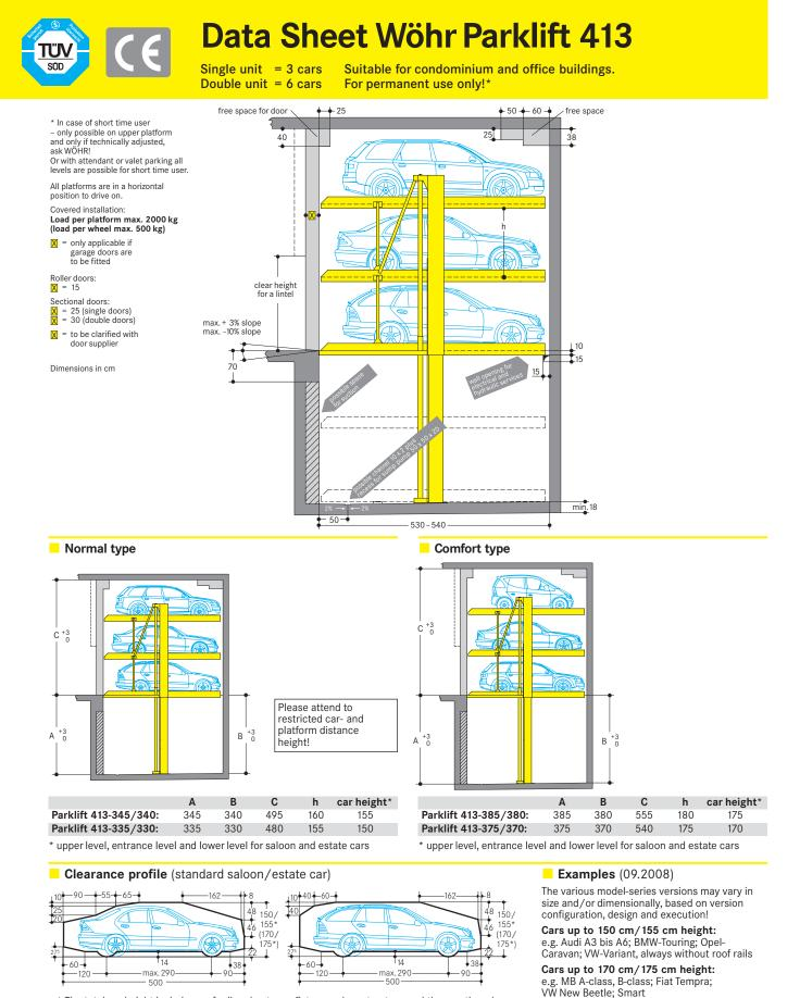
\* The total car height includes roof rail and antenna fixture and must not exceed the mentioned max. height dimension.
