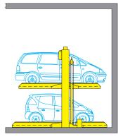
Before lowering the platforms, the car on the entrance level must be driven off!
