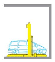
Before lowering the upper platform, the car on the middle level must also be driven off!
