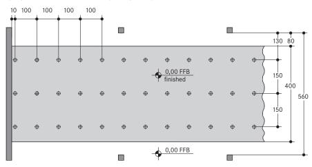
Measuring points at 100 cm points for checking unevenness acc. to DIN 18202, table 3, line 2, or acc. diagram
