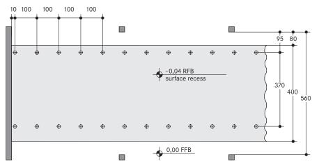
Measuring points at 100 cm points for checking unevenness acc. to DIN 18202, table 3, line 2, or acc. diagram
