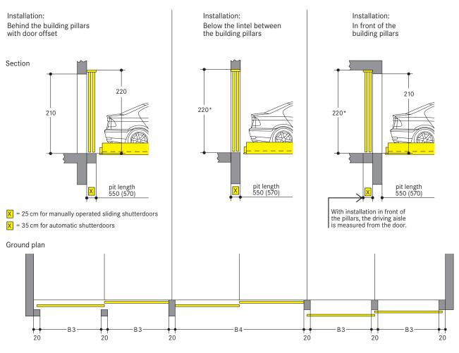
\* The lintel of 220 cm is absolutely necessary. If differing heights additional fixings are required at additional charge. If no lintel is provided, the gates need to be fitted onto a steel frame (subject to surcharges).
